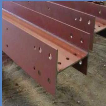
**Structural steel** components are engineered specifically for the building location. The main frame steel will vary in size and there is really no limit to the size of the frame. Used for the largest span buildings.
