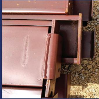
Structural steel has a painted finish typically in red although can come in many colors. The paint is intended only to protect the steel during construction and transport and is easily damaged.
